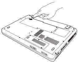
(Sample Illustration) Locking the battery release lock
